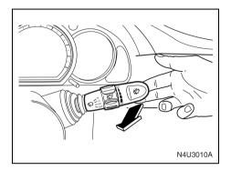
To wash your windshield, pull the windshield wiper/washer lever toward you with the ignition in the ON position.
